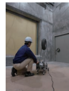
Floor-sound insulation testing led to SHAIDD55, our high-performance acoustic isolation floor system.
